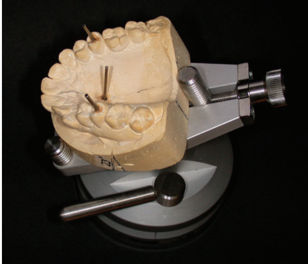
Figure 3 The working model mounted on an adjustable table and tilted by 23^\circ to the vertical plane (which is represented by the premolar rods). The implant rod enters the model at the distal level of the first premolars
